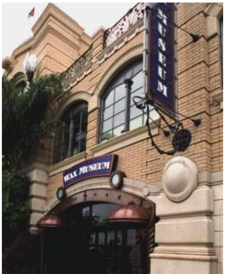
An architect's selection of stone can affect other building materials as well. Initial plans to completely clad the San Francisco Wax Museum in limestone went by the wayside due to cost; instead, limestone went into select fixtures, and limestone ingredients were included in materials such as cement plaster coatings.
